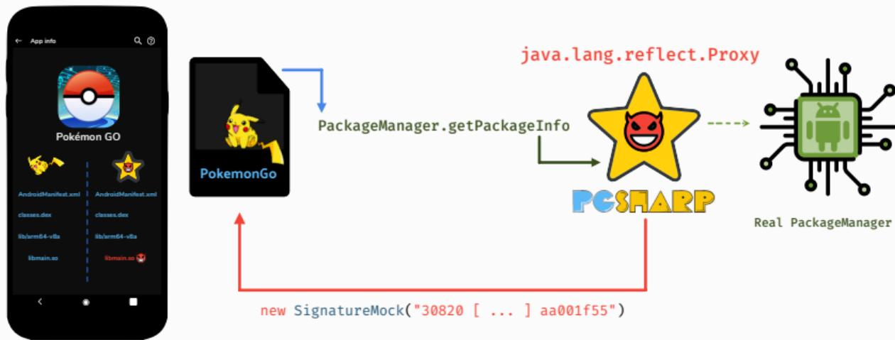
Figure 1: Signature bypass based on a proxy of the Android PackageManager
